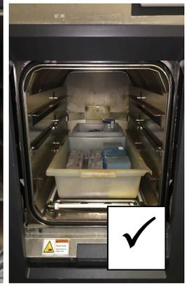
D) Appropriate plastic secondary containers are properly placed inside the autoclave equipment.
