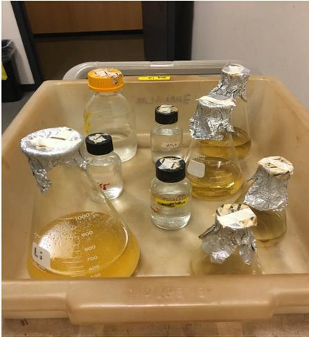
A) Pyrex flasks are filled to only 75% of their holding capacity and placed inside appropriate plastic secondary container, with space between each item to allow steam to circulate.
