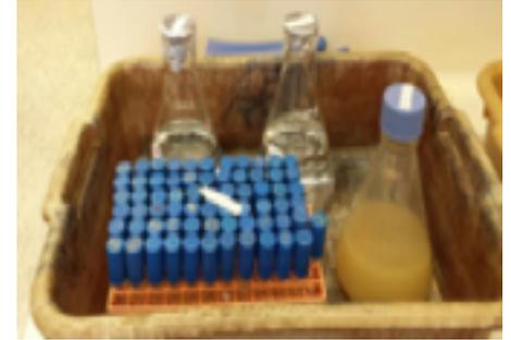
B) 75% filled primary items are spaced in appropriate plastic secondary container.
